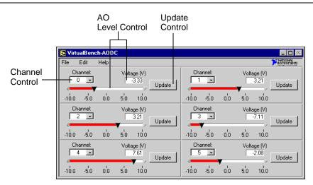
The front panel of VirtualBench-AODC has the following features:
